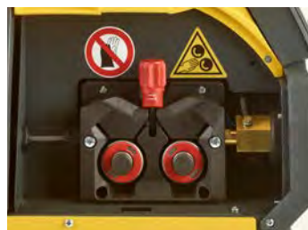
Professional double groove feeding mechanism with 4 rolls
