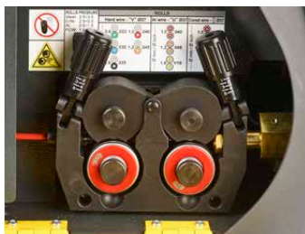
Professional double groove feeding mechanism with 4 rolls
