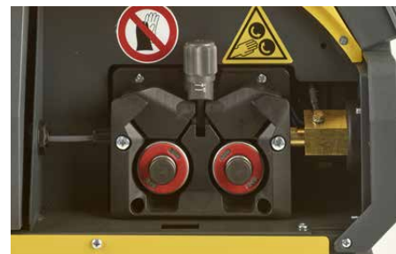
Professional double groove feeding mechanism with 4 rolls
