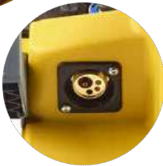
INCLINED TORCH CONNECTION
